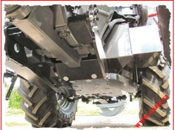
JAKE Aid Frame goes under the tank reducing the clearance around 8 cm. Material thickness of the tank bottom is around 3 mm.
