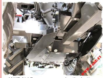
JAKE Aid Frame goes under the battery case reducing the clearance around 8 cm. Armour thickness is 5 mm.
