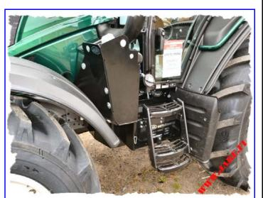
AdBlue-tank is lifted as up as possible and covered by 5 mm thick steel. Under the staircase is an armoured and lockable tool box. Original staircase mudguard is usable.
